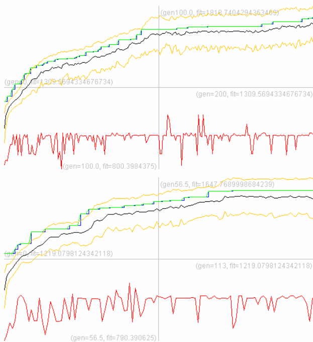
Fig. 2: Elitist algorithm with E = 0.3 , C = 0.22 in generation 110; E = 0.3 , C = 0.22 in generation 200; E = 0.3 , C = 0 in generation 110; and E = 0.3 , C = 0 in generation 200 (from top to bottom). X-axis is generation number, Y-axis is fitness. Red is the least fitness in a generation, green is top fitness in a generation, blue is best fitness up-to-date, black is average generation fitness, orange is average fitness + standard deviation.
